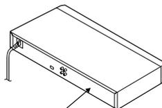
The rating plate and the safety caution are on the rear of the unit.
