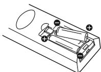
Make sure to match the + and – on the batteries to the marks inside the battery compartment.
