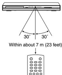
Distance: About 7 m (23 feet) from the front of the remote sensor
