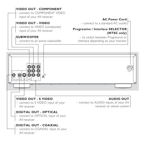
Caution: Do not touch the inner pins of the jacks on the rear panel. Electrostatic discharge may cause permanent damage to the player.
