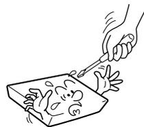
c) Never short-circuit the battery pack by either accidentally or intentionally bringing the terminals in contact with another metal object. This could cause personal injury or a fire, and could also damage the battery pack.
