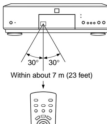
Distance: About 7 m (23 feet) from the front of the remote sensor
