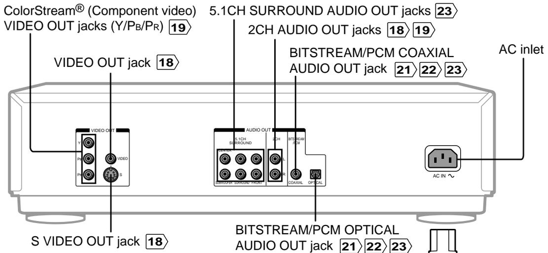
When connecting the optical digital cable, remove the cap and fit the connector into the jack firmly. When not using the jack, keep the cap inserted to protect it from dust intrusion.
