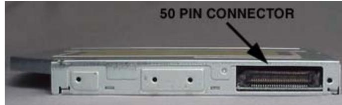
**Figure 1. SD-C2512 DVD Writeable Drive Rear Panel – Connector**
