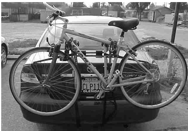
Fig. 7: On a bike with a slanted top tube, place top tube on rear cradle, and down tube on front cradle to keep bike as “level” as possible.
