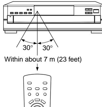
Distance: About 7 m (23 feet) from the front of the remote sensor
