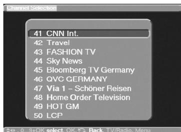
If the receiver is in TV mode, only TV programmes will be shown, and in Radio mode only radio programmes will be displayed. The programme currently selected is highlighted in red.
