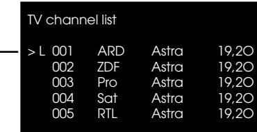
Example: how to change channel 3, Pro 7, with channel 4, Sat 1
