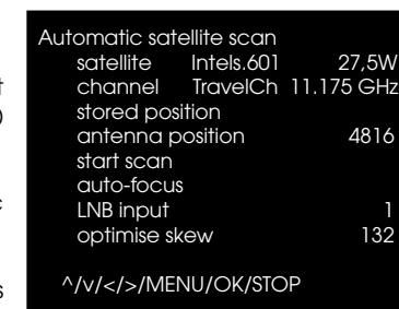
Press **◀** to switch over to the next satellite West (Intelsat 601 at 27.5° West in our example).
