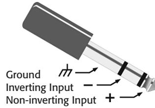
**Unbalanced Inputs:** Connect to the plug as shown. If a 3 conductor (TRS) plug is used to connect an unbalanced source, Pin 3 and pin 1 must be connected with a jumper as shown.
