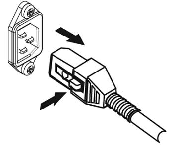
The K Series is fed by a universal power supply. This power supply is capable of operating the system with input AC power voltages ranging from 85 VAC to 265 VAC at 50 – 60 Hz. There are multiple power cables supplied for this reason.
