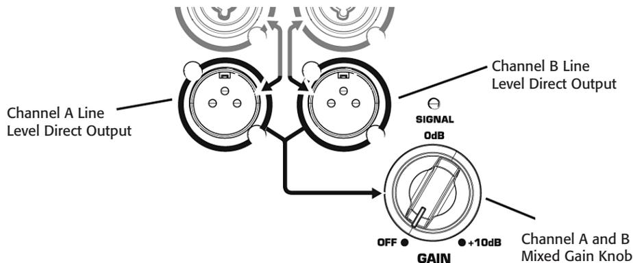
Both Channel A and Channel B have discrete direct outputs on female XLR connectors. The signal on this output is exactly equivalent to the signal from the corresponding input. The level of the output signal is not affected by the gain set on the subwoofer gain knob.
