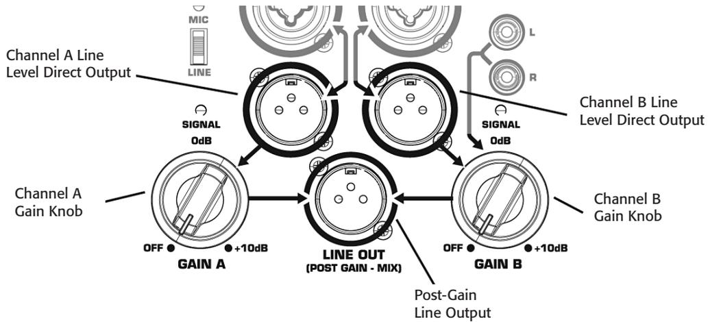
Both Channel A and Channel B have discrete direct outputs on female XLR connectors. The signal on this output is exactly equivalent to the signal from the corresponding input. The level of the output signal is not affected by the gain setting for that channel. Additionally, signal delivered on the RCA (phono) jacks is not present on the Channel B direct line level output.
