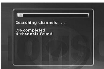
An installation window will appear. A cursor shows the progress in the set-up of the channels. When all the channels that you can receive in your area have been stored, **100 %** is indicated. Press **OK** to return to the **Channel search** line. Press **MENU** to return to the Main Menu.
