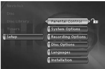
Note: the padlock tells you whether or not the DTH 8005 is locked. When the **Lock** function is activated, a padlock is displayed on the DTH 8005 display.
