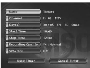
*Note: your DTH 8005 can memorise the parameters of 16 different programmings. In the case of double programming, a warning message is displayed.*
