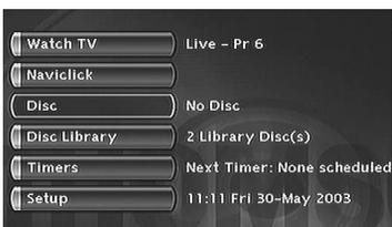
Note: the **Disc** heading is shown as transparent when there is no disc in the device or if the disc is not compatible.
