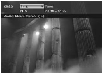
Note: when the information banner is displayed at the top of the screen you have the possibility of choosing an audio channel (if this is provided by the channel) using the **➤** key on the remote control. To display information again, press the **INFO** key of the remote control.
