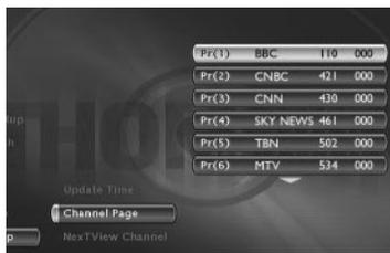
*Note: For correct operation of the Naviclick guide described on page 25, it is indispensable that a Teletext page number (for those channels broadcasting it) is indicated for each channel. The page numbers allocated to channels on this screen were set during the installation of your DTH 8005. We recommend that you do not change them.*
