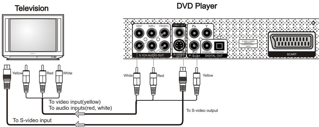
If the TV-set has S-video input, the DVD player can be connected with an S-video cable. When using an S-video cable, don't use the yellow video cable.
