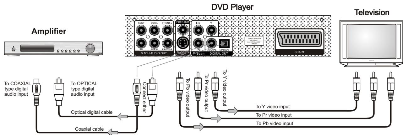
If the receiver is provided with coaxial input, the DVD player can be connected with a coaxial cable. When a coaxial cable is used, don't use the optic cable.
