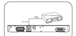
To listen the sound from your VCR, TV or Satellite Receiver through the speakers of this unit, only connect the Left / Right audio output of these equipments to the
