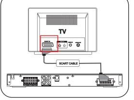
To view the video from DVD disc on your TV set, connect the TV SCART OUT jack of this unit to the SCART jack of your TV set using a scart cable
