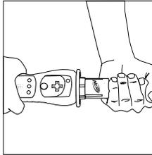
4) Double check that the Locking Collar is firmly affixed to the Sports Handle Attachment-Head. Apply extra clockwise twist to make sure no more rotation is possible.
