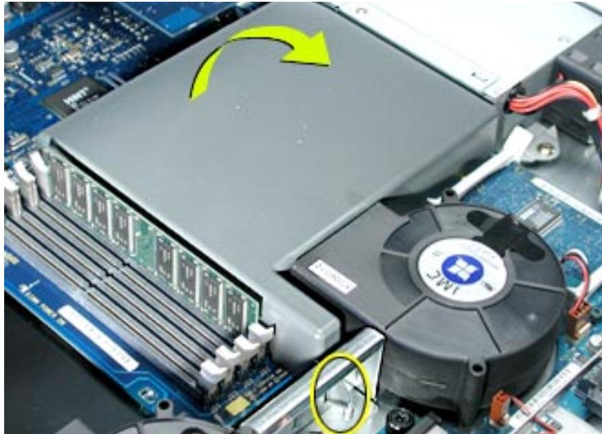
3. If necessary, disconnect the blower cable nearest the ATA controller board. **(Figure 4)**
