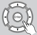
**Use the [▲]/[▼] buttons to select the parameters, press the [Enter] button, and use the [◀]/[▶] buttons to set them.**
