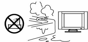
**19. Clean only with dry cloth**---Unplug this product from the wall outlet before cleaning. Do not use liquid cleaners or aerosol cleaners. Use a damp cloth for cleaning.
