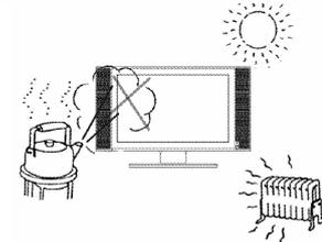
**22. Panel protection**---The LCD panel used in this product is made of glass. Therefore, it can break when the product is dropped or impacted upon by
