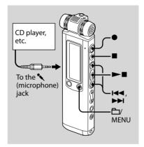
You can make music files without using the computer by recording the sound from other equipment, such as a CD player, connected to the IC recorder. When you use the synchronized recording function, the IC recorder enters the recording pause mode when no sound is detected for more than 2 seconds and the IC recorder starts recording again as a new message when sound is detected.
