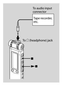
To record the sound of the IC recorder with other equipment, connect the
