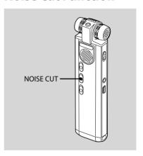
When the NOISE CUT switch is set to "ON," the distortion of very low and high frequencies which are outside the human voice range is reduced, therefore you can hear the human voice more clearly.
