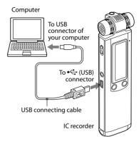
While the batteries are charging, "CONNECTING" and the battery indicator are displayed in an animation.
