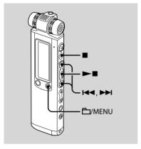
When you set the LCF (Low Cut Filter) function to "ON" in the stop or recording mode, you cut out a frequency of lower than 200 Hz to reduce the roaring noise from wind, etc., this helps to record a sound source more clearly.
