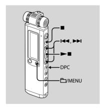
When you slide the DPC (Digital Pitch Control) switch to "ON," you can adjust the playback speed between +200% and -75% of normal speed in the menu. The message is played back in natural tones by the digital processing function.
