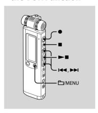
You can set the VOR (Voice Operated Recording) function to "ON," to make the IC recorder start recording when the IC recorder detects sound, and pause when no sound is heard, eliminating recording during soundless periods.
