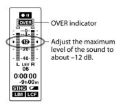
Press and hold ◄ or ► to change the sound level continuously. The sound level is also displayed as a number below the level meter.
