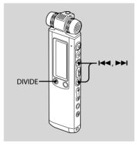
You can divide a message during playback, so that the message is divided into two parts and a new message number is added to the newer part of the divided message. By dividing a message, you can easily find the point from which you want to play back when you make a long recording such as at a meeting. You can divide a message until the total number of messages in the folder reaches 999 or until the
