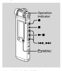
When "ADD/OVERWRITE" in the menu is set to "OVERWRITE," you can add an overwrite recording after a selected point in a recorded message. The part of the message after the selected point is deleted.
