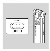
When you are not using the IC recorder, you can prevent the batteries from getting weak quickly by turning the power off.
