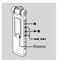
During the stop or recording mode set "LIMITER" to "ON," and the input level is set automatically within the maximum input level to prevent the sound distortion which occurs when a sound that is too loud is input. A sound that is too loud
