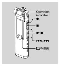
When "ADD/OVERWRITE" in the menu is set to "ADD," you can add a recording to the message being played back. The added recording will be placed after the current message, and will be counted as a part of the message.
