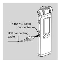
You can charge the rechargeable batteries by connecting the IC recorder to an AC outlet using a USB AC adaptor AC-U50A (not supplied).
