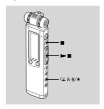
1 During playback, press ⊊ (repeat) A-B/★ to specify the starting point A.
