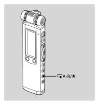
You can add priority marks (★) to important messages. There are four levels, "★★\*" (the most important), "★★," and no priority mark. You can add priority marks both in the stop mode, and in the playback mode.
