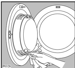
Clean periodically the interior part of the door to remove any fluff. Accurate cleaning ensures correct drying.
