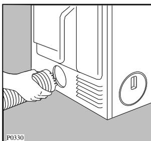
Remove the collar by pulling it out of the vent outlet. Screw the collar to the vent hose. Fit the hose into the required vent outlet, and place vent covers provided over the unused outlets.
