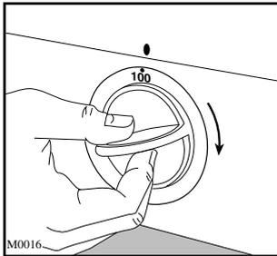
Turn the selector dial clockwise to the required minute setting (in the high or low temperature range, according to the fabric): the mains-on light illuminates and the machine starts operating.
