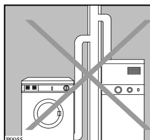
You should **NOT** connect the flexible vent hose to, for example, a chimney or flue pipe designed to carry the exhaust from a fuel burning heating appliance.
