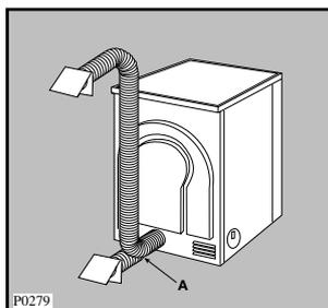
The vent hose must not contain more than two bends when it is placed in position for operation.
