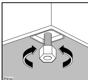
Level the tumble dryer into place by screwing or unscrewing the front feet as required.
