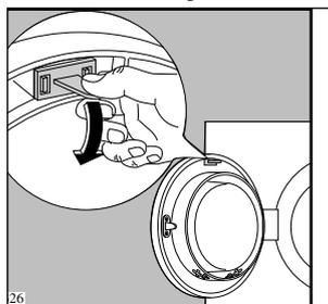
This tumble dryer incorporates a special child safety feature. At the top, on the inside of the porthole door, you will notice a catch, if this is removed it will prevent the machine from working. To remove, press the catch downwards (see picture). You **MUST** replace the catch to enable the appliance to work.
