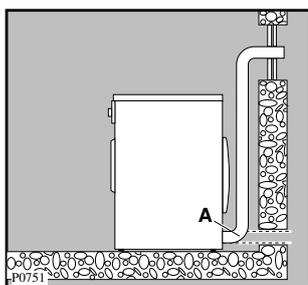
Connect the other end of the hose to an opening in a door or window. Fit a suitable shield or point the hose downwards to prevent any rain water and wind from getting in.
