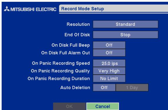
Figure 45 — Record Mode Setup screen.
