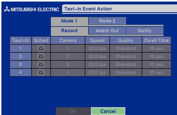
Figure 55 — Text-In Event Action (Record) setup screen.
