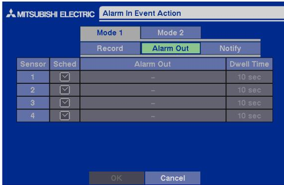
Figure 50 — Alarm In Event Action (Alarm Out) setup screen.
