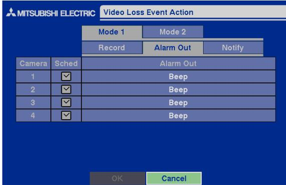
Figure 59 — Video Loss Event Action (Alarm Out) setup screen.
