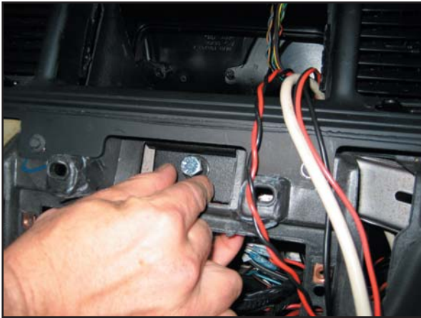
Attach #2 bracket to dash frame with 3/8" hex bolt, washers, and nut.
