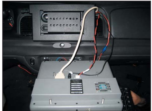
Attach computer wiring and monitor adaptor bracket.
