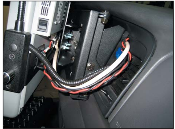
Position and wire tie wiring.
