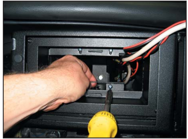
Attach top & bottom dash clamps (#3 bracket) with #8x1" phillips machine screws.
