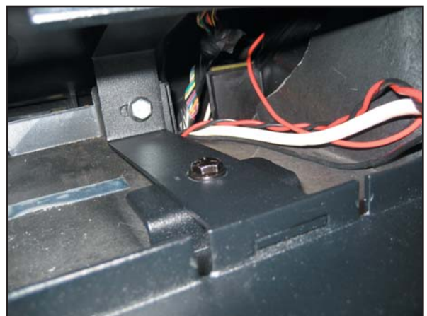
Attach monitor mount to #1 and #2 brackets with 1/4" bolts provided.
