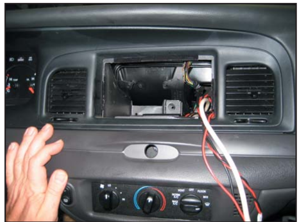
Reattach center dash trim and run computer wires.
