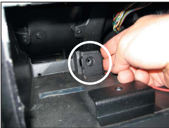
Slip #1 bracket over plastic AM/FM radio support.
