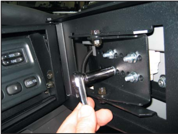
Attach monitor bracket to dash mount with 1/4" nuts.
