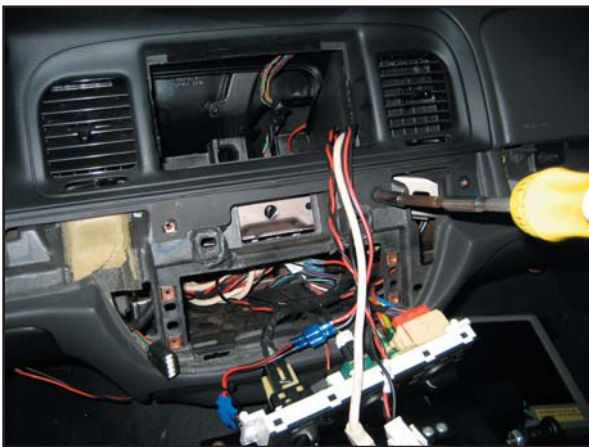
Remove 4 screws at lower end of the upper dash panel. (7mm socket)
