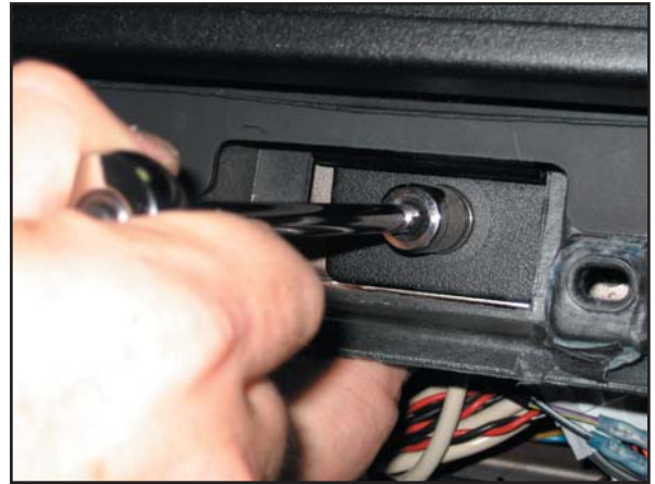
Tighten 3/8 bolt. (9/16 socket and wrench)
