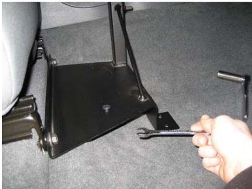
Tighten "Z" bracket to base assembly.
