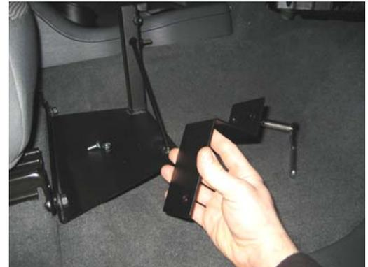
Install "Z" support bracket to base assembly using  $\frac{1}{4}$  x  $\frac{3}{4}$ " carriage bolt and serrated nut.
