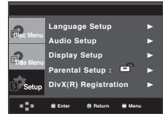
3. Press the **▲/▼** buttons to select **Parental Setup**, then press the **▶** or **ENTER** button.
