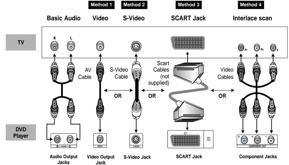
1. Connect a cable with the desired method.
