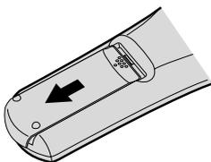
2 Install two "AAA" batteries observing the correct polarity as shown in compartment.
