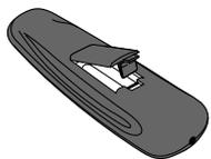
1. Remove the battery compartment cover.
