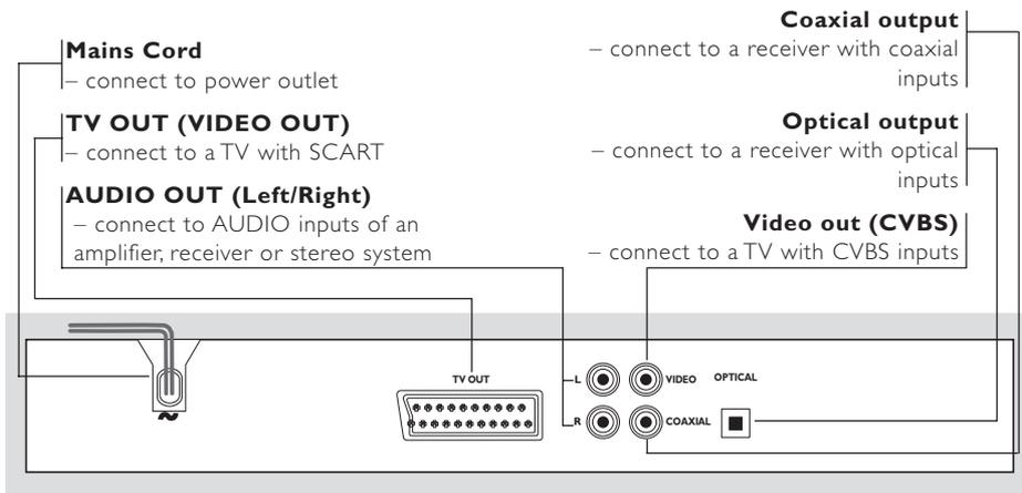
**Caution: Do not touch the inner pins of the sockets on the rear panel. Electrostatic discharge may cause permanent damage to the unit.**
