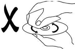
Do not wipe in a circular direction (Concentric scratches in the disc groove tend to cause noise.) Gently wipe from the inside to the outer edge.
