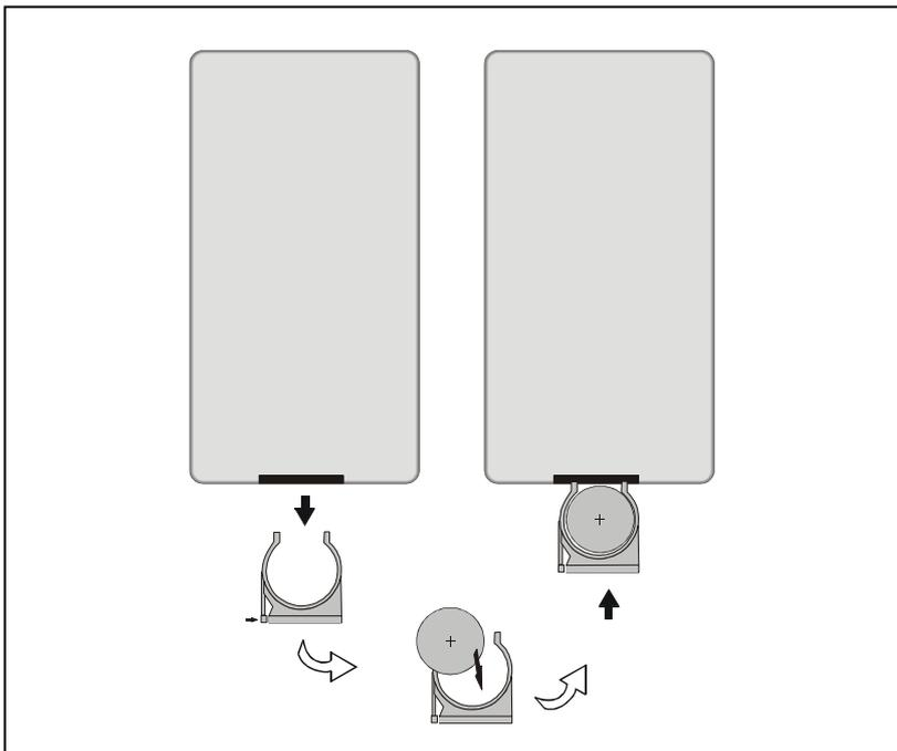
1. Refer to the drawing, take the back cover off of the remote control and remove the empty battery receptacle.
