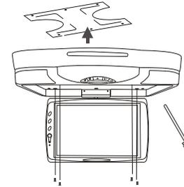
4. Flip the monitor screen down and tighten the monitor to the support bracket, using the supplied screws.
