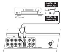
For an optical connection, use an optical cable (not supplied) to connect the **OPTICAL DIGITAL AUDIO OUT** jack to an optical input on your AV receiver.
