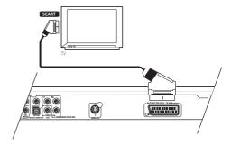
1 Use a SCART cable (not supplied) to connect the AV CONNECTOR (RGB) output to a SCART AV input on your TV (or AV receiver).
