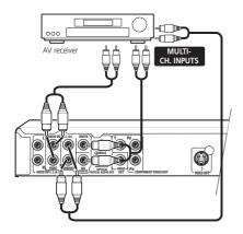
You can use the SCART AV connector, or the S-video or component video jacks to connect to the AV receiver if you prefer.
