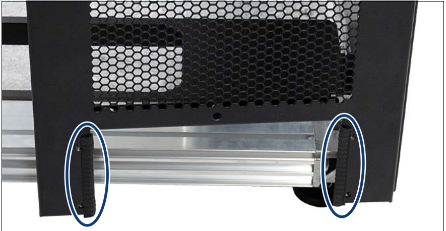
Figure 18: Cable cut-out with edge protectors
