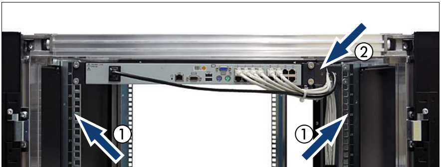
Figure 13: Example of how to mount a rack component in the 19-inch area at the back
