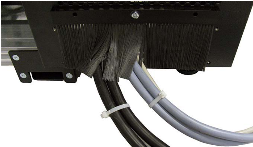
Figure 20: Cables leaving the rack through the cat door
