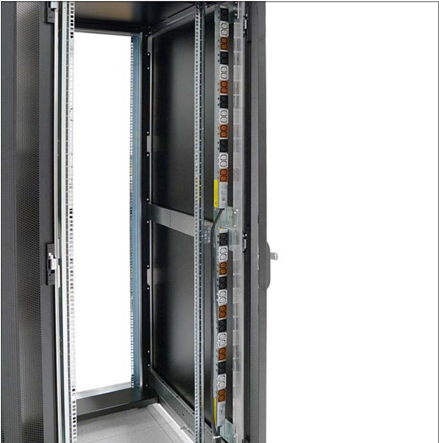
Figure 55: 3-phase socket strip w/ 3x8 sockets mounted 2x in a 700 mm wide symmetrical rack
