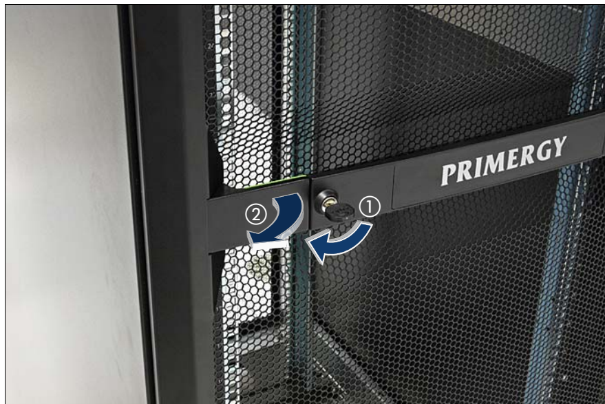
Figure 6: Opening the rack door
