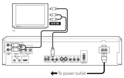
The setup described here is a basic setup that allows you to play discs using just the cables supplied with the player. In this setup, stereo audio is played through your TV.
