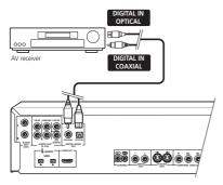
Optical connection: Use an optical cable (not supplied) to connect the OPTICAL DIGITAL AUDIO OUT jack to an optical input on your AV receiver.
