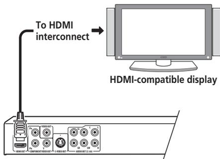
The arrow on the cable connector body should be face up for correct alignment with the connector on the player.
