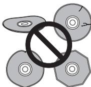
This player is designed to be used only with conventional, fully circular discs. Do not use shaped discs. Pioneer disclaims all liability arising in connection with the use of shaped discs.
