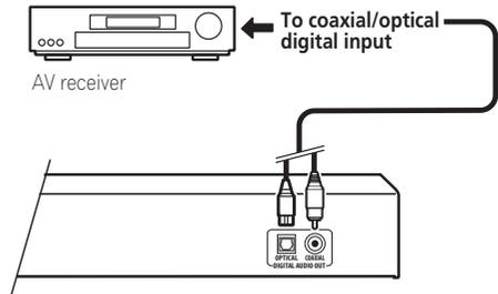
For an optical connection, use an optical cable (not supplied) to connect the **OPTICAL DIGITAL AUDIO OUT** jack to an optical input on your AV receiver.
