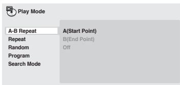
**2 Press ENTER on 'A(Start Point)' to set the loop start point.**
