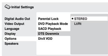
If you've selected **DTS > PCM** in *DTS Out* on page 39 or **2 Channel** in *Audio Output Mode* on page 45, you can choose the way the signal is downmixed to PCM audio. **STEREO** will downmix the DTS signal to 2-channel stereo, whereas **Lt/Rt** will downmix to a 2-channel signal compatible with Dolby surround matrix decoders. (This allows you to hear surround sound if your AV receiver or amplifier has Dolby Pro Logic capability.)
