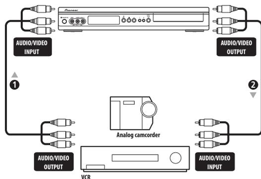
**1 Connect a set of audio and video outputs of your VCR or camcorder to a set of inputs on this recorder.** This enables you to record tapes from your VCR or camcorder.
