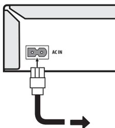
**1 Use the supplied power cable to connect this recorder to a power outlet.**
