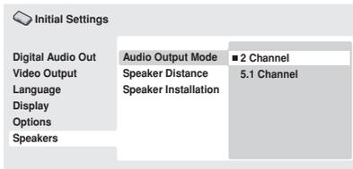
If you connected this player to your amplifier using the 5.1 channel analog outputs (front, surround, center and subwoofer outs), set this to **5.1 Channel**; if you connected only the stereo outs, set to **2 Channel**.
