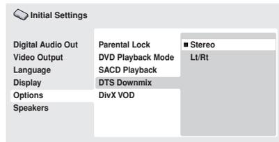
If you've selected **DTS > PCM** in *DTS Out* on page 34 or **2 Channel** in *Audio Output Mode* on page 40, you can choose the way the signal is downmixed to PCM audio. **Stereo** will downmix the DTS signal to 2-channel stereo, whereas **Lt/Rt** will downmix to a 2-channel signal compatible with Dolby surround matrix decoders. (This allows you to hear surround sound if your AV receiver or amplifier has Dolby Pro Logic capability.)
