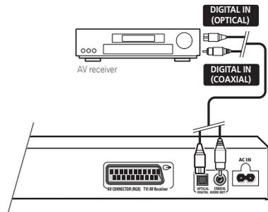
For an optical connection, use an optical cable (not supplied) to connect the **OPTICAL DIGITAL AUDIO OUT** jack to an optical input on your AV receiver.
