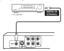
Use a coaxial cable (similar to the supplied video cable) to connect the **COAXIAL DIGITAL AUDIO OUT** jack to a coaxial input on your AV receiver.
