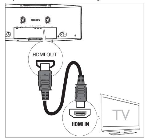
Connect HDMI (High Definition Multimedia Interface), DVI (Digital Visual Interface), or HDCP (High-bandwidth Digital Contents Protection)-compliant TVs through HDMI for the best picture quality. This connection transmits both video and audio signals. Through this connection, you can watch DVDs that contain HD (High-Definition) content.
