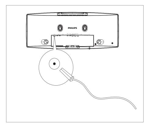
1 Connect the supplied FM antenna to the FM AERIAL socket on the unit.
