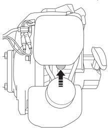
Choke: Set the choke control in the choke position.
