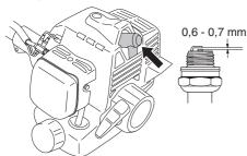
**CAUTION!** Always use the recommended spark plug type! Use of the wrong spark plug can damage the piston/cylinder. Check that the spark plug is fitted with a suppressor.
