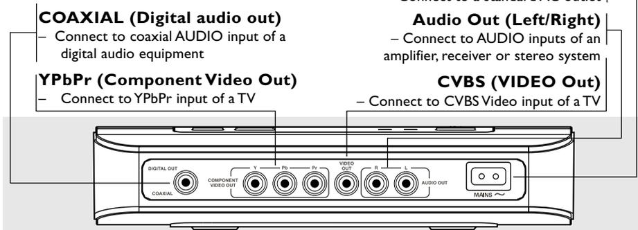
**Caution: Do not touch the inner pins of the jacks on the rear panel. Electrostatic discharge may cause permanent damage to the unit.**
