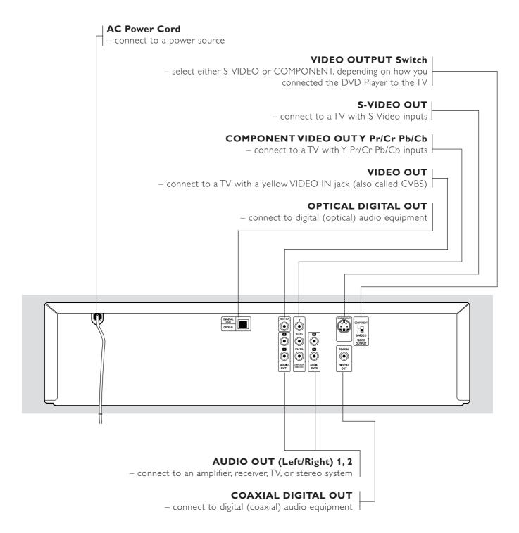
Caution: Do not touch the inner pins of the jacks on the rear panel. Electrostatic discharge may cause permanent damage to the unit.
