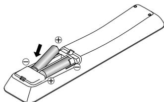
Make sure to match + and - on the batteries to the marks indicated in the battery compartment.
