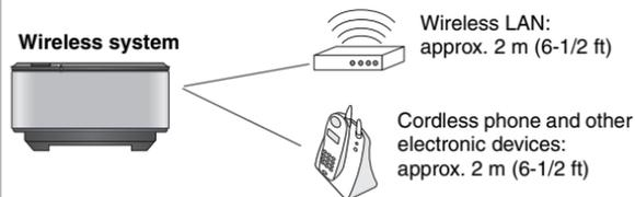
The wireless system will automatically seek a clear channel if any of these other devices interfere with its communication. When this happens, the wireless link indicator ("W1" or an indicator) flashes on the home theater unit, and there is a brief interruption in audio coming from the surround speakers.
