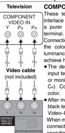
**COMPONENT VIDEO OUT terminals** These terminals can be used for either interlace or progressive output and provide a purer picture than the S-VIDEO OUT
