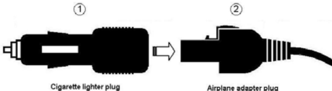
(b) In an airplane, insert directly the airplane adapter plug into a plane's in-seat power receptacle.
