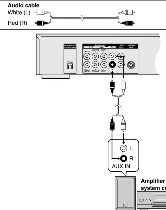
**D** Connecting a digital amplifier or system component
