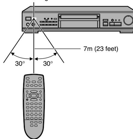
Aim at the sensor, avoiding obstacles, at a maximum range of 7 m (23 feet) directly in front of the unit.
