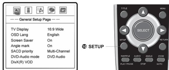
2. Press the LEFT/RIGHT ARROW buttons to select the setup page. There are 5 pages: **General Setup**, **Speaker Setup**, **Audio Setup**, **Video Setup**, and **Preference**. Press the SELECT button to enter the selected setup page. The **Preference** page can only be accessed when playback is completely stopped, or when there is no disc in the player.
