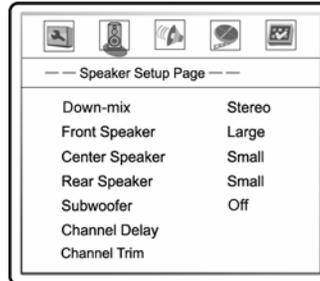
1. **Down-mix Mode:** This sets the audio down-mix mode to convert multi-channel audio into two-channel output. This setting only affects the “Mixed L/R” analogue audio outputs. The options are:
