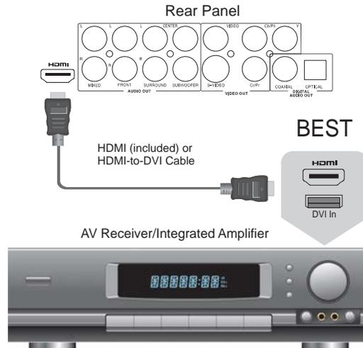
HDMI can transmit both audio AND video signals over a single cable. If you have an HDMI-capable display or, better yet, an HDMI-capable receiver that can support HDMI audio, you are in luck. Simply run an HDMI cable from the OPPO DVD player to your display or receiver and enable HDMI audio (if necessary) on that device (see your receiver or display’s owners’ manual for more information). You are now equipped to send all current audio formats to your display or receiver.
