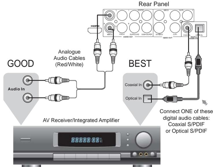
If at all possible you will want to connect audio using digital cables (either coaxial S/PDIF or optical S/PDIF). If your receiver or integrated amplifier does not have Dolby Digital or DTS capability (for instance, an older Pro Logic model) then you should connect the “Mixed” stereo output of the OPPO DVD player to your receiver or integrated amplifier (and immediately start saving for an upgrade!) Setting up, you have the following choices:
