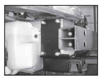
11. Install eight 3/8" x 1-1/4" bolts, 3/8" lock washers, and 3/8" hex nuts. Install bolts from inside outwards. We require that "LOCTITE. Blue" be used on all bolts.
