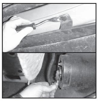
6. Remove two plastic push fasteners from bottom side of bumper and unplug fog light.
