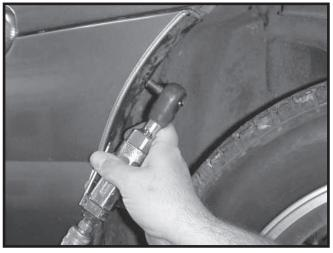
2. Remove screws from wheel well to facia on each side.
