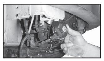
Bend horn bracket to clear base plate when installed.
