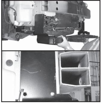
**9.** Slide base plate up from bottom and line up tight against front frame bracket as shown in picture. Clamp in place.
