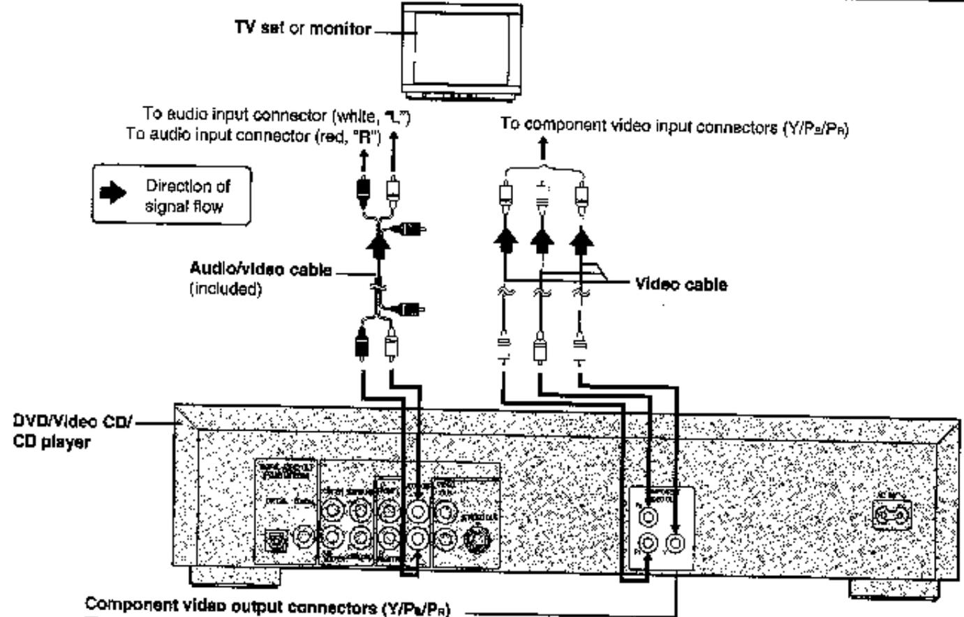
**Component video output connectors (Y/P<sub>B</sub>/P<sub>R</sub>)**
