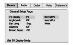
The TV Display which select the different ratio of display format and the screen of TV, There are various types of display on screen for different matches between Disc and TV (Please see page 20; Multi-image ratio mode)
