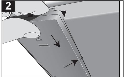
**TO REMOVE:** Press down the Battery Release button on the rear of the Battery Pack, then slide the Battery Pack out towards the rear of the unit.
