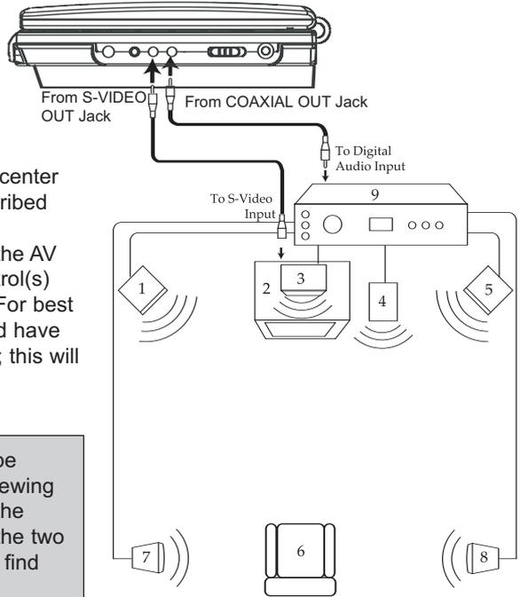
Place the subwoofer, front, rear and center speakers in locations as shown/described here. After correctly positioning the speakers, perform the Tone Test on the AV Amplifier and adjust the Volume control(s) until the desired sound is achieved. For best results, sit in the viewing position and have someone adjust the volumes for you; this will enable you to set the optimal levels.
